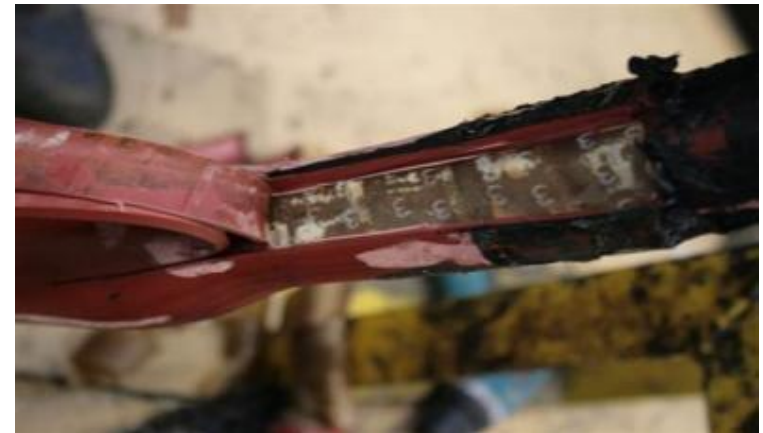
PD tracks on a dried PILC
